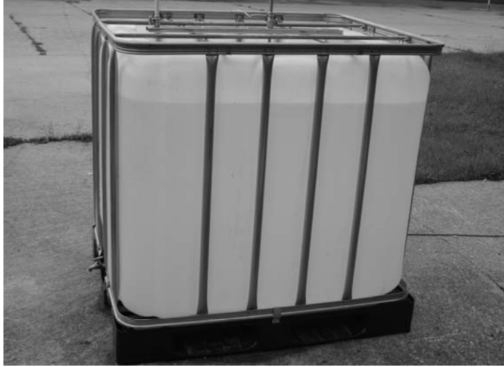
Fig.1. Tank with capacity of 1000 l
