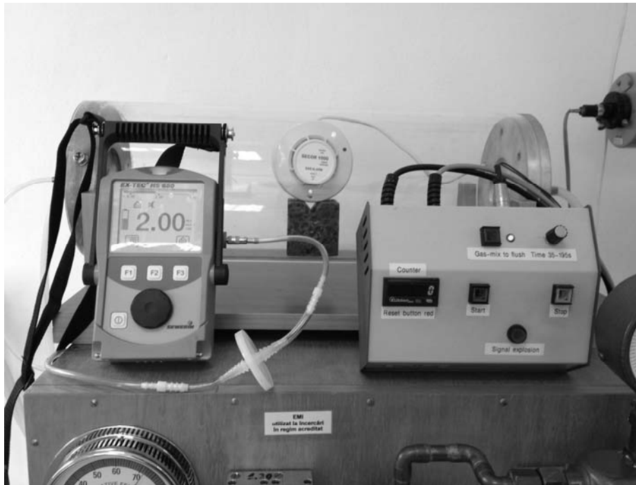
Fig. 1. Test rig for testing domestic gas detectors
